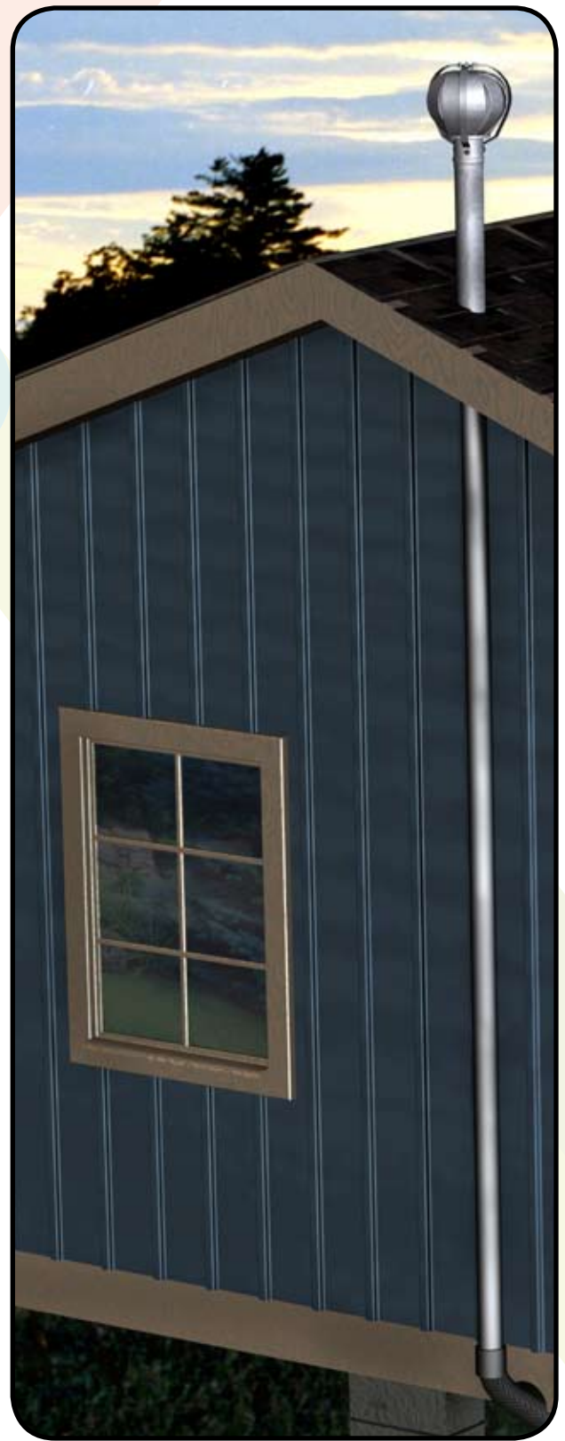
TYPICAL VENT UP SIDE WALL
